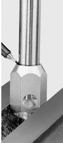
Figure 3-59 Marking the tube.
