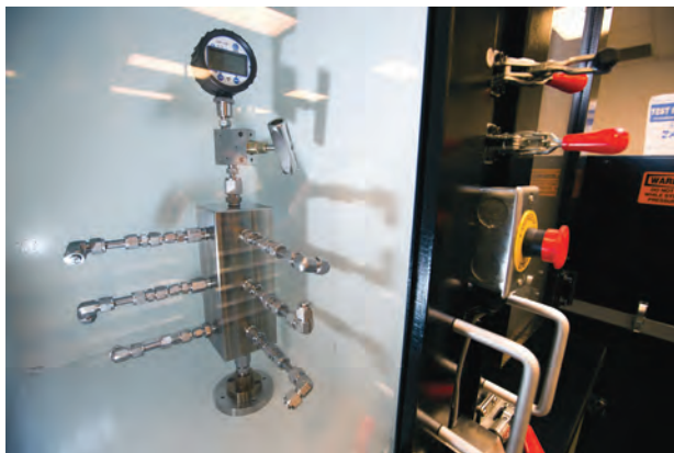
Figure 7-9 Hydraulic impulse test.
